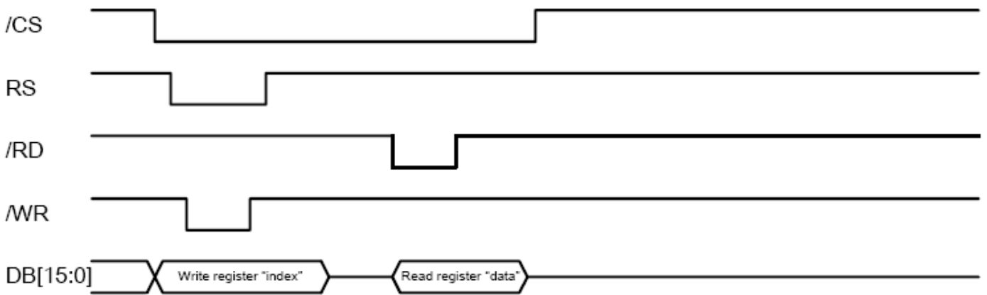
16-bit System Bus Interface Timing(Register Read Timing)
