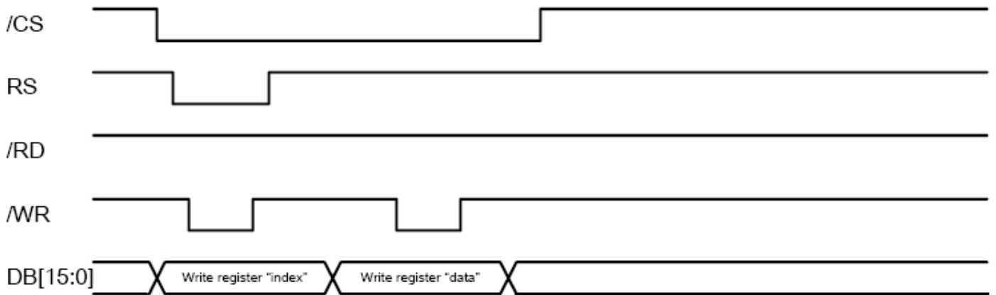
16-bit System Bus Interface Timing(Register Write Timing)
